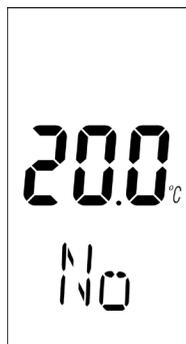
Timer Mode allows you to set a specific setpoint temperature for a period of time. The screen shows the image on the left.
